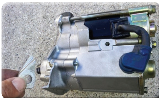
Broken mounting tab on cast aluminum bracket.
